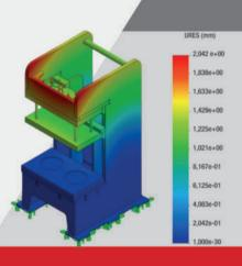
Static, structural and dynamic analyzes were performed out in the body design of the press. Side walls are manufactured from a single piece of sufficient thickness, without the use of welded reinforcements.
